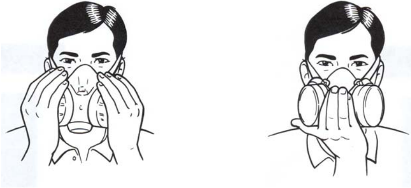
Figure 1 Negative pressure fit check Figure 2 Positive pressure fit check
